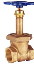
T/S-134 Rising Stem Gate Valve Class 150 BRZ Body, Union Bon- net Solid Wedge, Integral Seat Size 1/4" to 3", Threaded or Solder
