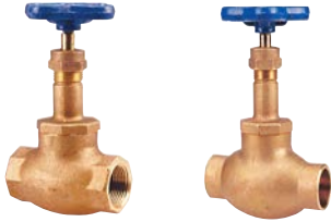
T/S-211 B/Y Globe Valve Class 125 BRZ Body, Screwed-In Bonnet, Bronze or TFE Disc Size 1/8" to 3", Threaded or Solder
