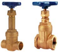
T/S-111 (T/S-113) Rising (N.R) Stem Gate Valve Class 125 BRZ Body, Screwed-In Bonnet, Solid Wedge, Size 1/4" to 3" Threaded or Solder
