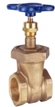
T/S-136 N.R. Stem Gate Valve Class 150 BRZ Body, Union Bonnet Solid or Split Wedge, Integral Seat Size 1/4" to 3", Threaded or Solder
