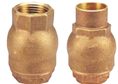
T/S-480-Y Lift Check Valve Class 125 Bronze Body Buna-N or TFE Disc Size 3/8" to 2", Threaded or Solder
