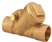
T/S-413-B/Y/W/V Swing Check Class 125 Bronze Body TFE, Buna-N or Viton Disc Size 1/2" to 2", Threaded or Solder
