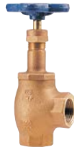
T/S 311 Angle Valve Class 125 BRZ body, Screwed in Bonnet, TFE Disc, Integral Seat Size 1/4" to 3" Threaded
