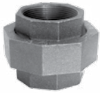
Fig. 463 Class 150 Union Size Range: 1/8" thru 3" Page 32
