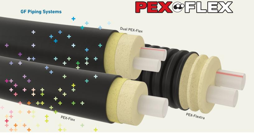
**PEX-Flex** is a pre-insulated pipe system complete with bonded polyurethane foam insulation and extruded polyethylene jacket. It is ideally suited for hydronic heating applications including campus style district energy, snow/ice melt systems and alternative fuel boilers such as outdoor wood furnaces. Supplied in coils and available with core PEX up to 4" single and 2" dual pipe, this seamless pipe system is economical, simple to install and highly effective even in harsh soil conditions.
