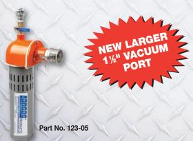
The Lansas Super-Vac<sup>™</sup> is a lower cost alternative for manhole vacuum testing. The new Super-Vac<sup>™</sup> will pull over 40 CFM @ 10" of mercury. The Super-Vac<sup>™</sup> will deliver more than 50% more volume than others on the market. The unit has no moving parts nor does it require any maintenance. Maximum vacuum is reached with an air source producing 80 CFM or better.
