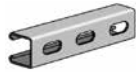
AS 400EH Channel with Elongated Holes Size: 1 5 / 8 " x 1" x 12 GA. 9/16" x 1 1 / 8 " Elongated Holes on 2" Centers.
