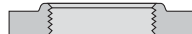
Fig. 1011 – Cast Iron Companion Flange Size Range: Fig. 1011: ¾" x 3/8" thru 12" x 19" NPS
