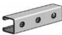
AS 520H Channel with Holes Size: 1 5 / 8 " x 1 3 / 16 " x 12 GA. 9/16" Holes on 1 7 / 8 " Centers.
