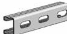
AS 560EH Channel with Elongated Holes Size: 1 5 / 8 " x 1 3 / 16 " x 16 GA. 9/16" x 1 1 / 8 " Elongated Holes on 2" Centers.
