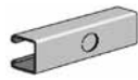
AS 400KO Channel with Knock Outs Size: 1 5 / 8 " x 1" x 12 GA. 7/8" Knock Outs on 6" Centers.
