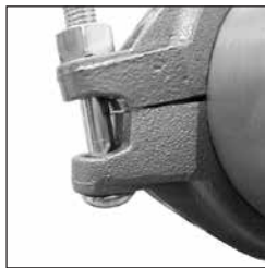
Excess Torque or Shallow Groove Dimension
