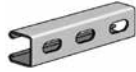
AS 500EH Channel with Elongated Holes Size: 1 5 / 8 " x 1 3 / 16 " x 14 GA. 9/16" x 1 1 / 8 " Elongated Holes on 2" Centers.
