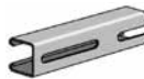
AS 520S Channel with Long Slots Size: 1 5 / 8 " x 1 3 / 16 " x 12 GA. 1 3 / 32 " x 3" Slots on 4" Centers.
