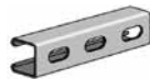
AS 520EH Channel with Elongated Holes Size: 1 5 / 8 " x 1 3 / 16 " x 12 GA. 9/16" x 1 1 / 8 " Elongated Holes on 2" Centers.
