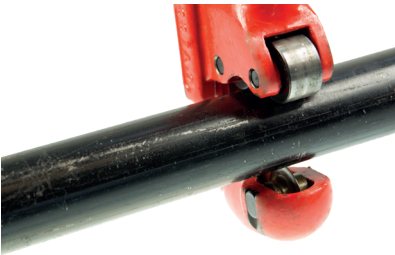
FIGURE 6: CUTTING THE PIPE
