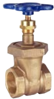
T/S-136 N.R. Stem Gate Valve Class 150 BRZ Body, Union Bonnet Solid or Split Wedge, Size 1/4" to 3", Threaded or Solder
