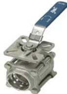
B05S SERIES 3 pc, full port, CF8M body, 316SS ball and stem, S.W, RTFE seats and seals, locking lever handle, ISO direct mount Size ½" to 4" 1000 PSI
