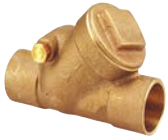
T/S-413-B/Y/W/V Swing Check Class 125 Bronze Body TFE, Buna-N or Viton Disc 1/2" - 2", Threaded or Solder
