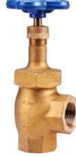
T/S 335Y Angle Valve Class 150 BRZ body, Union Bonnet, TFE Disc, Integral Seat Size 1/8" to 3" Threaded
