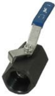
Flow+ B06 Series 1 PC REG. Port Carbon Steel 2000 PSI Ball Valve, FNPT Threaded on both ends. ASTM A105N Carbon Steel Size 1/4" to 2"
