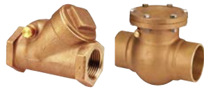
T/S-433-B/Y (S-433-B) Swing Check Class 150 Bronze Body Bronze or TFE Disc, 1/2" - 3" (4") Threaded or Solder
