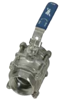
B04S SERIES 3 pc, full port, CF8M body, 316SS ball and stem, SW, RTFE seats and seals, locking lever handle Size ½" to 4" 1000 PSI
