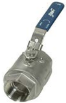
B01 SERIES 2 pc, full port, CF8M body, 316SS ball and stem, NPT, RTFE seats and seals, locking lever handle Handle Size ¼" to 2 ½" 1000 PSI
