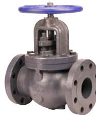
F-768-B Globe Valve Class 250 C.I. Body Bolted Bonnet BRZ DISC, Size 2" to 8" FLG Connection
