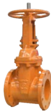
GTVA-FD3151-HW Gate Valve Class 125 D.I. Body, Resilient seated, OS & Y, Size 2" -12" FLG connection
