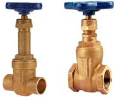
T/S-111 (T/S-113) Rising (N.R.) Stem Gate Valve Class 125 BRZ Body, Screwed-In Bonnet, Solid Wedge, Size 1/4" to 3" Threaded or Solder
