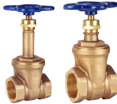
T-131 (T-133) Rising (N.R.) Stem Gate Valve Class 150 BRZ Body Screwed-In Bonnet, Solid Wedge Size 1/4" to 3", Threaded
