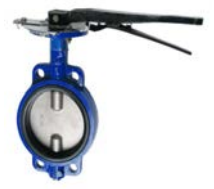
NCI/ Flow+ Wafer Style BFV, D.I. Body Elec. Plated DI Disc 304SS shaft, PTFE bearings EPDM seats Size 2" to 12" Lever or Gear
