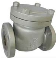
F-771-FR - F-774-FR Check Valve Class 150/300, WCB Body, OS&Y Bolted Bonnet Stellite HF Trim Size 2"-12", RF FLG Connection
