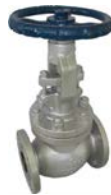
F-761-FR-F764-FR Globe Valve class 150/300 WCB Body, OS&Y Bolted Bonnet Stellite HF SEAT Size 2"-24", FLG Connection
