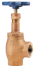
T/S 311 Angle Valve Class 125 BRZ body, Screwed in Bonnet, TFE Disc, Integral Seat Size 1/4" to 3"
