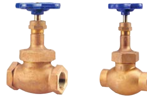
T/S-235Y Globe Valve Class 150 BRZ Body, Union Bonnet TFE Disc, Integral Seat 600 CWP, Size 1/4" to 2" 400 CWP, Size 2 1/2" to 4"
