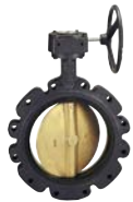
WD5022 / LD5022 BFV Wafer / Lug Style 285 PSI D.I. Body, Molded-in Liner, S.S. Disc Size 2" - 12"
