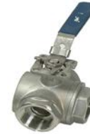
B07T-B07L SERIES 3 way, CF8M body, 90 degree T-port or L Port 316SS ball and stem, NPT ends, RTFE seats and seals, locking lever handle, ISO direct mount Size ½" to 2" 1000 PSI
