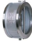
300WTCTB ( 300WTTTM / 300WTTTV) Class 300# Carbon Steel Body (Stainless steel body) - Wafer Connection - Stainless Disc - Buna Seat (Metal / Viton Seat) Size 4" to 12"
