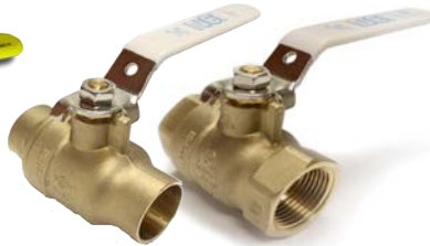
SFP600-LF TFP600-LF 2 PC Brass Ball Valve FP600 LF LEAD FREE 600 CWP, Size 1/4" to 2" 400 CWP, Size 2 1/2" to 4" Threaded or Solder
