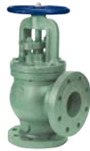
F-838-31 Globe Valve D.I Angle Valve Class 150, D.I Body, Bolted Bonnet BRZ Disc, Size 2"-8", FLG Connection
