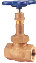
T-275-AP Globe Valve Class 300 BRZ Body, Union Bonnet Stainless Steel Disc & Seat 600 CWP, Size 1/4" to 2" 400 CWP, Size 2 1/2" to 4" Threaded or Solder
