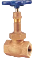
T-275-B/Y Globe Valve Class 300 BRZ Body, Union Bonnet BRZ or TFE Disc & Bronze Seat 600 CWP, Size 1/4" to 2" 400 CWP, Size 2 1/2" to 4" Threaded or Solder
