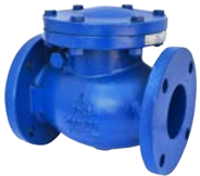
CKVA-FCI1330 SWING CHECK Class 125 C.I. Body, C.I. DISC, BRZ OR C.I. Mounted Seat Size 2-1/2" to 12" FLG Connection
