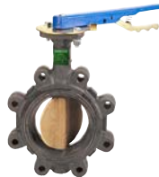
WD3000 BFV Wafer Style, 250 PSI, D.I. Body Molded-in Liner D.I., S.S. or Alum. Brz. Disc Size 2" - 12"
