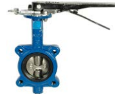
NCI/Flow+ Lug Style BFV C.I. Body 316SS DISC, 304 SS Shaft EPDM seat Size 2" to 12" Lever or Gear
