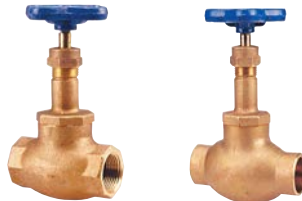
T/S-211 B/Y Globe Valve Class 125 BRZ Body, Screwed-In Bonnet, Bronze or TFE Disc 600 CWP, Size 1/4" to 2" 400 CWP, Size 2 1/2" to 4"
