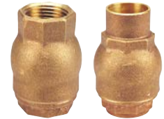
T/S-480-Y Lift Check Valve Class 125 Bronze Body Buna-N or TFE Disc 3/8" - 2", Threaded or Solder
