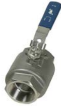
B02 SERIES 2 pc, full port, CF8M body, 316SS ball and stem, NPT ends, RTFE seats and seals, locking lever handle, actuator mounting pad 2000 PSI to 1-1/4" & 1500 PSI 1-1/2" & 2"
