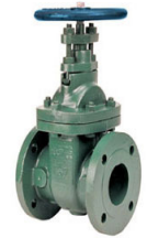
F-639-31/33 Gate valve Class 150 D.I Body, N.R.S Bolted Bonnet, BRZ/SS Mounted Trim, Solid Wedge, Size 2" - 16" RF.FLG Connection
