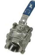
B04 SERIES 3 pc, full port, CF8M body, 316SS ball and stem, NPT, RTFE seats and seals, locking lever handle Size ½" to 4" 1000 PSI
