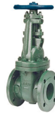
F-637-31/33 Gate valve Class 150 D.I Body, OS&Y Bolted Bonnet, BRZ/SS Mounted Trim, Solid Wedge, Size 2" - 24" RF. FLG Connection
