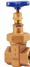
T-176SS A.N.R. Stem Gate Valve BRZ Body, Union Bonnet Solid BRZ or Alloy Wedge, BRZ or SS Seat. Size 1/4" to 2" Threaded
