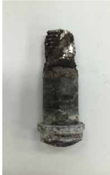
Hardened White Substance Coating Majority of Interior Body, Stem, Ball & Seat Damaged Beyond Repair
